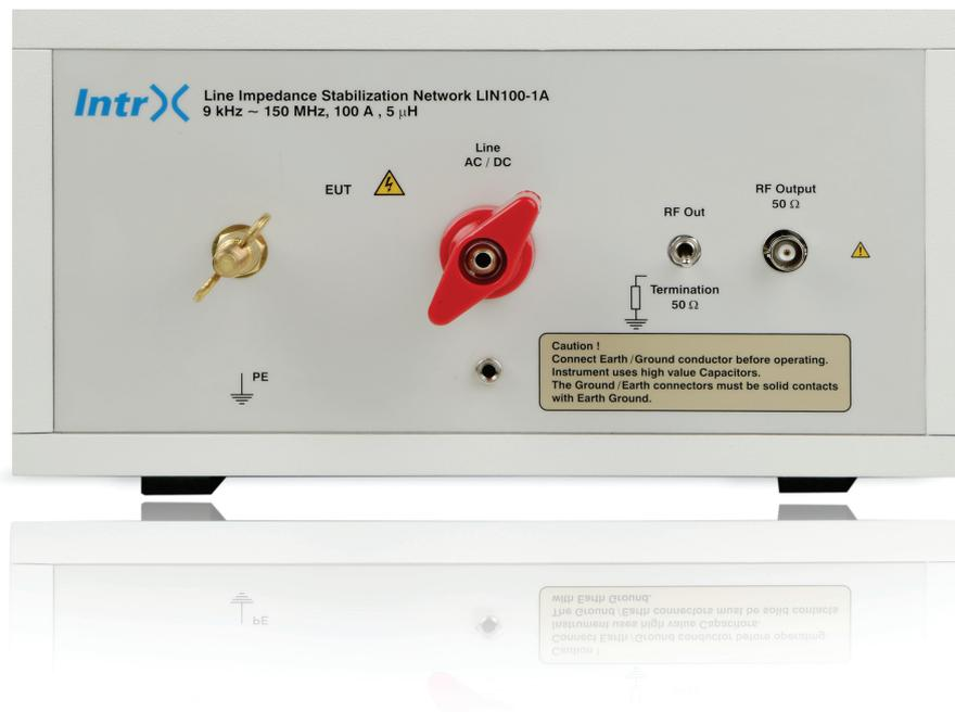
LISN (Artificial Mains Network) is a low-pass filter typically placed between an AC or DC power source and the EUT (Equipment Under Test) to create a known impedance as per complying standard for the measurement of conducted emission. It also isolates the unwanted RF signals from the power source with pre-filter included. It provides a Radio frequency (RF) noise measurement port.
